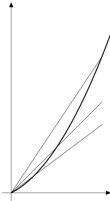
Figure 42: The slope at a point as the limit of the slopes of secant lines.
