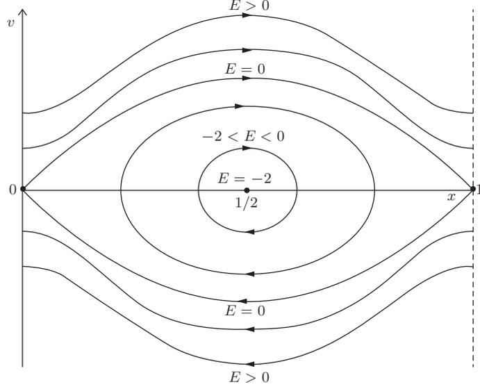
FIGURE 3. The phase space of the simple pendulum.
