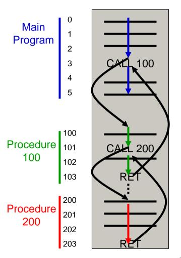
The stack can be used also to pass parameters to the called procedure
