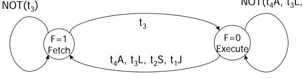
• There is just one boolean expression for the transition condition of the unique state variable  $F_{n+1} = F_n t_3' + F_n' t_4 A + F_n' t_3 L + F_n' t_2 S + F_n' t_1 J$
