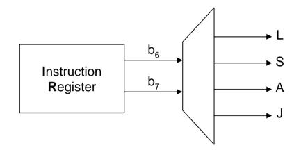
Inside the Control Unit a 2-to-4 decoder provides L, S, A, J signals denoting which instruction is currently in IR
