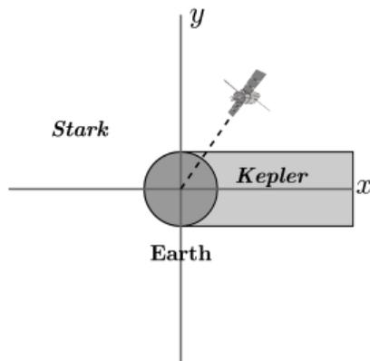
The Sun-shadow dynamics is a model to study the short-period evolution of an Earth satellite subjected to the solar radiation pressure which passes through the Earth shadow. It arises by patching two integrable dynamics: Kepler's and Stark's dynamics.
