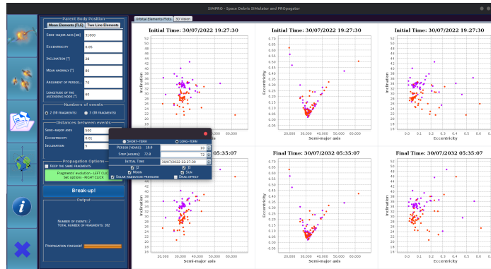
FIGURE C.3: Screenshot of the SIMPRO application - the multiple break-up event window.
