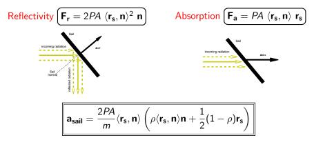
Where, if  $\rho$  is the reflectivity coefficient and *a* is the absorption coefficient, then  $\rho + a = 1$  (Notice that  $\rho = 0$  corresponds to a solar-panel and  $\rho = 1$  to a perfectly reflecting solar sail).
