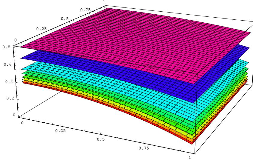
**Fig. 3** State  $y$  of the Dirichlet boundary control problem using the objective functional  $J(y, u) = \frac{1}{2} \|y - y_*\|_{H^s(\Gamma_y)}^2 + \frac{1}{2} \|u\|_{H^{1/2}(\Gamma)}^2$  for  $s = 0.1, 0.2, 0.3, 0.4, 0.5, 0.7, 0.9$  (from bottom to top) on resolution level  $J = 5$ .
