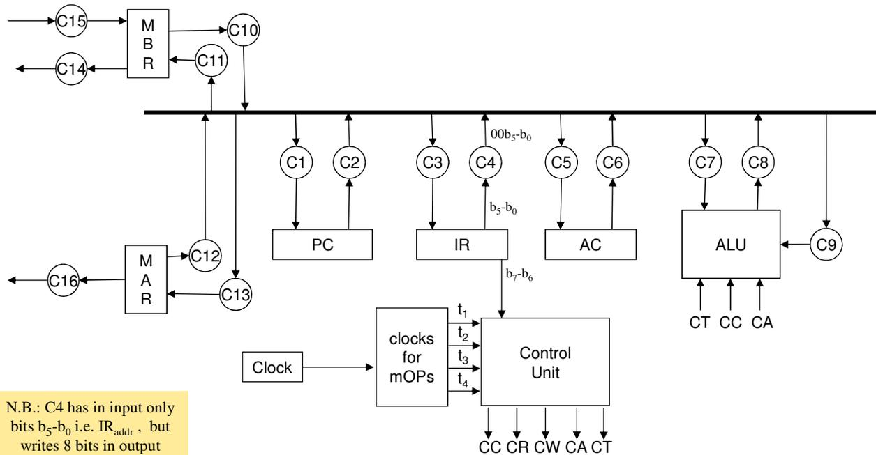
N.B.: C4 has in input only bits  $b_5-b_0$  i.e.  $IR_{addr}$ , but writes 8 bits in output
