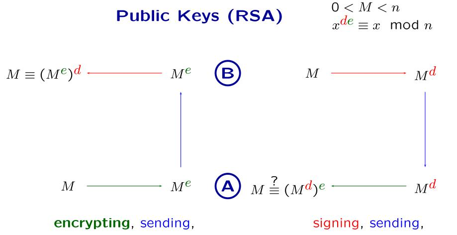
and decrypting and decrypting a message M signing, sending, and checking the signature of a message
