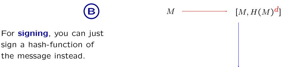
$$(A) \stackrel{?}{\equiv} (H(M)^{d})^{e} \longleftarrow [M, H(M)^{d}]$$
