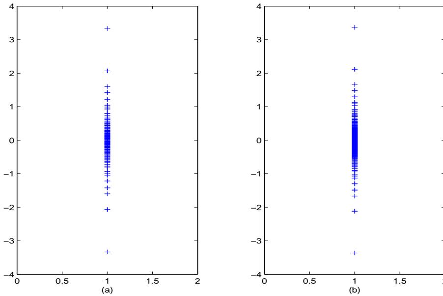
FIG. 4.1. Eigenvalues for the preconditioned problem with  $\nu = 1/30$ ,  $a = 1$ , discretization in two dimensions using centered differences and  $q = [-\sqrt{2}/2 \quad \sqrt{2}/2]^T$ . (a)  $h = 1/16$ ; (b)  $h = 1/32$ ,  $h$  stepsize.
